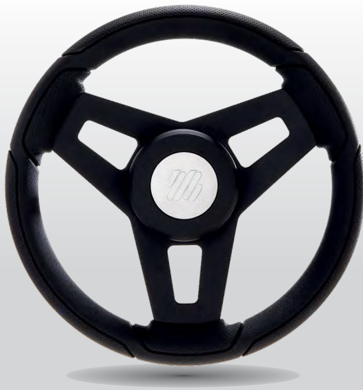
Montecristo PU B/B/CH 20351V Ø 350 mm (13.8") - Depth: 98 mm (3.86") Black polyurethane grip, black aluminum spokes, black painted cover
