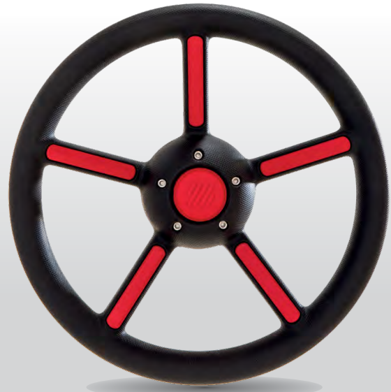
V56 B/R 21524F Ø 350 mm (13.8") - Depth: 95 mm (3.74") Black polyurethane grip and spokes with red painted inserts
