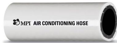
Specially formulated for chiller circulation and drain lines in air conditioning systems. Extra heavy-duty white PVC cover with black PVC inner tube reinforced with braided polyester yarn. Superior kink resistance. Temperature range is -40°F to 150°F (-40°C to 66°C).
