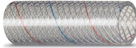
Clear Reinforced PVC Tubing (Red & Blue Tracer) Excellent for use in potable water, as well as hot and cold pressurized water applications. Heavy-duty clear vinyl, non-toxic reinforced tubing produced with an odorless and tasteless FDA approved compound. Not recommended for use with alcohol, petrochemical, or solvents. Operating temperature range -20°F to 150°F. (-29°F to 66°F).
