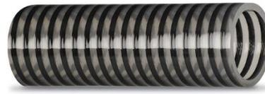
For use in heavy-duty bilge pump discharge and livewell circulation. Smooth clear PVC tube reinforced with black PVC helical rod for excellent flexibility. Clear smooth outer surface permits easy clamping and visual inspection of blockage. Not recommended for use in alcohol, anti-freeze, petrochemical, mild acid, solvent or pressurized water systems. Temperature range is -40°F to 160°F (-40°C to 71°C).
