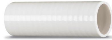
Smooth wall extra heavy-duty vinyl hose with PVC helical reinforcement. Has the same flexibility as our Premium Sanitation Hose. Extra odor fighting compound for all head and holding tank connections. Not recommended for use in alcohol, anti-freeze, petrochemical, potable water, solvent or pressurized water systems. Temperature range is -40°F to 160°F (-40°C to 71°C).
