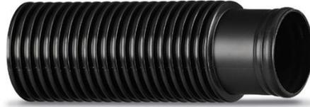
Ideal for electric and manual bilge pumps and livewell aerators. Heavy-corrugated polyethylene construction with custom molded cuff every foot for easy installation and clamping. Excellent flexibility. Resists heat, cold, sea water, ozone and oily bilge acids.
