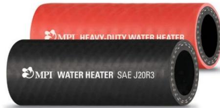
Used mainly for engine water, water heater, air conditioning circulation, icebox, sink and shower drain lines. Heavy EPDM tube and cover reinforced with high-strength polyester yarn. Resistant to mild chemicals, heat, cold, ozone and sea water. Temperature range is -40°F to 210°F (-40°C to 99°C).
