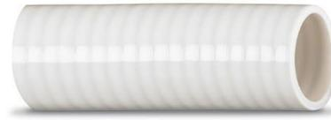
FDA approved compounds. For use in holding tank connection, sanitation vent and toilet systems. Smooth extra heavy-duty PVC tube, reinforced with PVC helical rod. Made with specially formulated FDA approved material to provide excellent resistance to odor permeation and toilet chemicals. Not recommended for use in Alcohol, anti-freeze, petrochemical, potable water, solvent or pressurized water systems. Temperature range is -40°F to 160°F (-40°C to 71°C).
