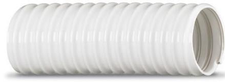
Extremely flexible vinyl hose supported by vinyl coated helical steel wire. Nylon reinforcement added to 1-1/2" I.D. hose for added strength. For use as heavy-duty bilge discharge and various drain lines. Temperature range is -40°F to 160°F (-40°C to 71°C).
